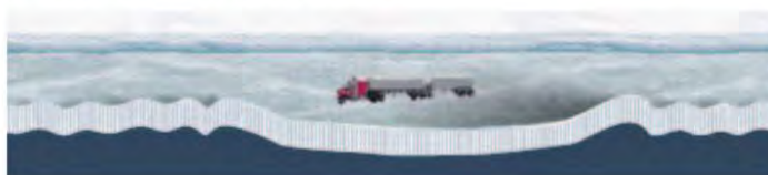
A fast-moving vehicle causes the ice to bend and creates dynamic waves in the ice ahead and behind the vehicle
