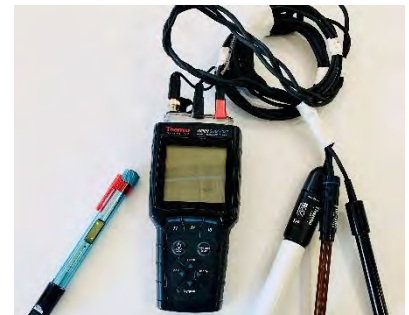
These probes can be used to measure water parameters like pH, oxygenation, and conductivity.
