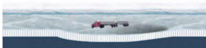
A slow-moving vehicle causes the ice to bend and forms a deflection bowl under the vehicle
