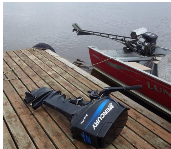
COMMON OUTBOARD MOTOR IS REPLACED BY A JET MOTOR TO NAVIGATE BETTER IN SHALLOW WATER AND REDUCE DAMAGE
