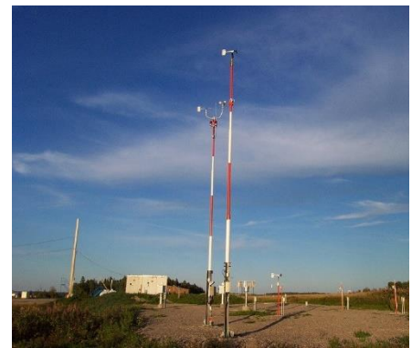
This automated weather station, located in Neskantaga, Ontario, measures temperature, dew point, humidity, wind, precipitation, and snow depth.
