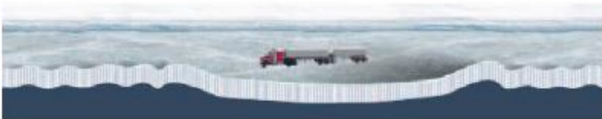
A fast-moving vehicle causes the ice to bend and creates dynamic waves in the ice ahead and behind the vehicle
